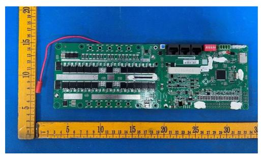
Figure 10. Front view of Main control PCB Board
