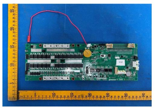
Figure 11. Back view of Main control PCB Board
