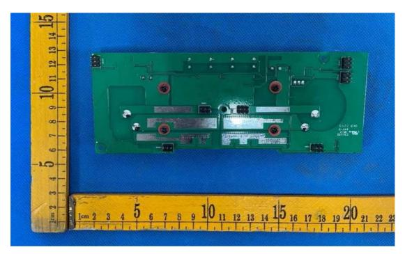
Figure 13. Back view of Current limit PCB Board
